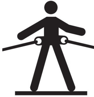
Figure 5 Pictogram illustrating application of a Class P work positioning full body harness
