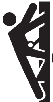
Figure 4 Pictogram illustrating application of a Class L ladder climbing access full body harness
