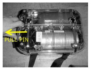
Step 2 – Lift and pull each latch ring (2) to release bands.
