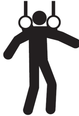
Figure 3 Pictogram illustrating application of a Class E limited access full body harness
