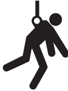
Figure 1 Pictogram illustrating application of a Class A fall arrest full body harness
