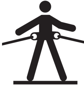
Figure 5 Pictogram illustrating application of a Class P work positioning full body harness
